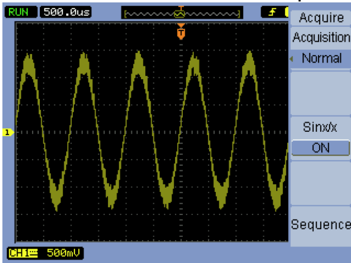
Noisy Waveform Without Averaging
