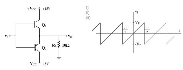
i) Assume the transistors are ideal with  $V_{BE1}=V_{EB2}=0$  V and  $V_{CEsat1}=V_{ECsat2}=0$ , for the input voltage  $v_I$  given above, plot the output waveform. (Assume  $V_P < V_{CC}$ )
