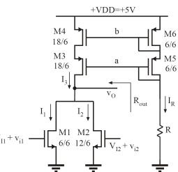
**3.** Consider the following current mirrors. This current mirrors are to be used as current sources.
