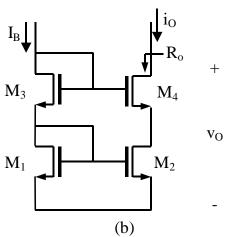
**4.** In the Wilson current mirror shown, assume the transistors' parameters are
