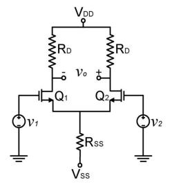
**2.** Consider the differential amplifier given in the figure below.
