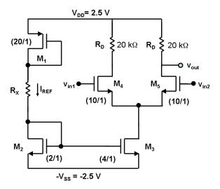
a) Determine the value of  $R_X$  to set  $I_{REF}$  = 100 $\mu$ A. Determine the drain current values for transistors  $M_4$  and  $M_5$ .
